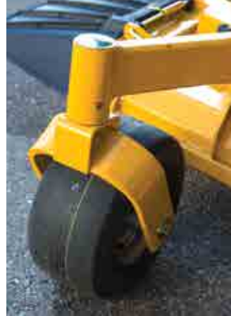
FRONT CASTER WHEELS WITH MOUNTED TAPERED GREASEABLE BEARINGS
