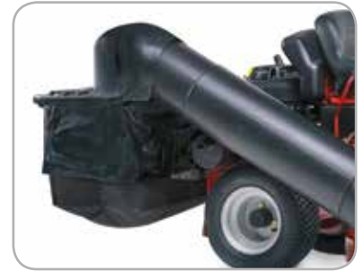
Single Bag Collector Accessible collection drawer with 175 litre capacity.
