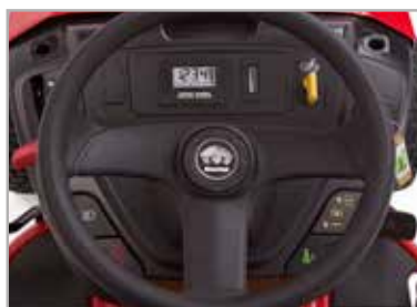
Mini Dash with hour meter, battery voltage and maintenance reminder
