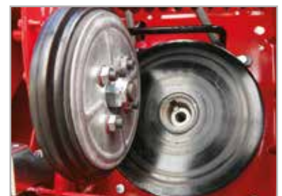
Variable speed disc drive transmission (RER)
