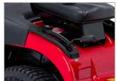
3,8 - 8,9 cm height-of-cut adjustable in 7 positions
