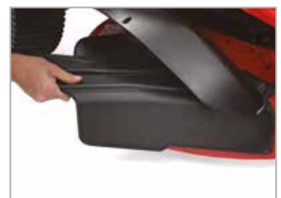
Toolless changeover from mulching to side discharge
