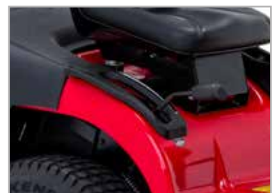
4,5 - 8,9 cm height-of-cut adjustable in 7 positions
