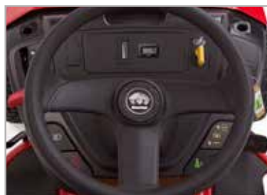
Ergonomically designed dash board with hour and fuel meter, cruise control
